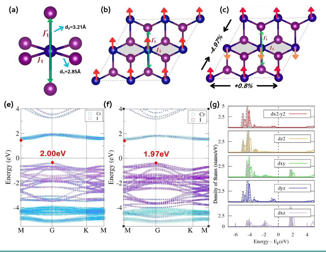
(c) To match the Crl<sub>2</sub> monolayer with In<sub>2</sub>Se<sub>3</sub> (lattice parameter a = 4.07Å), a biaxial strain was applied: +0.8% along the a direction (tensile) and -4.97% along the b direction (compressive).
